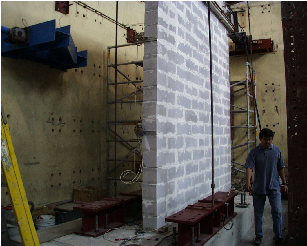
Figure 2.26: Side view of Shear Wall Specimen 18
