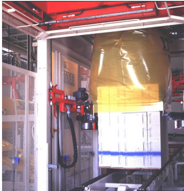
Figure B.7 Packaging of finished AAC units
