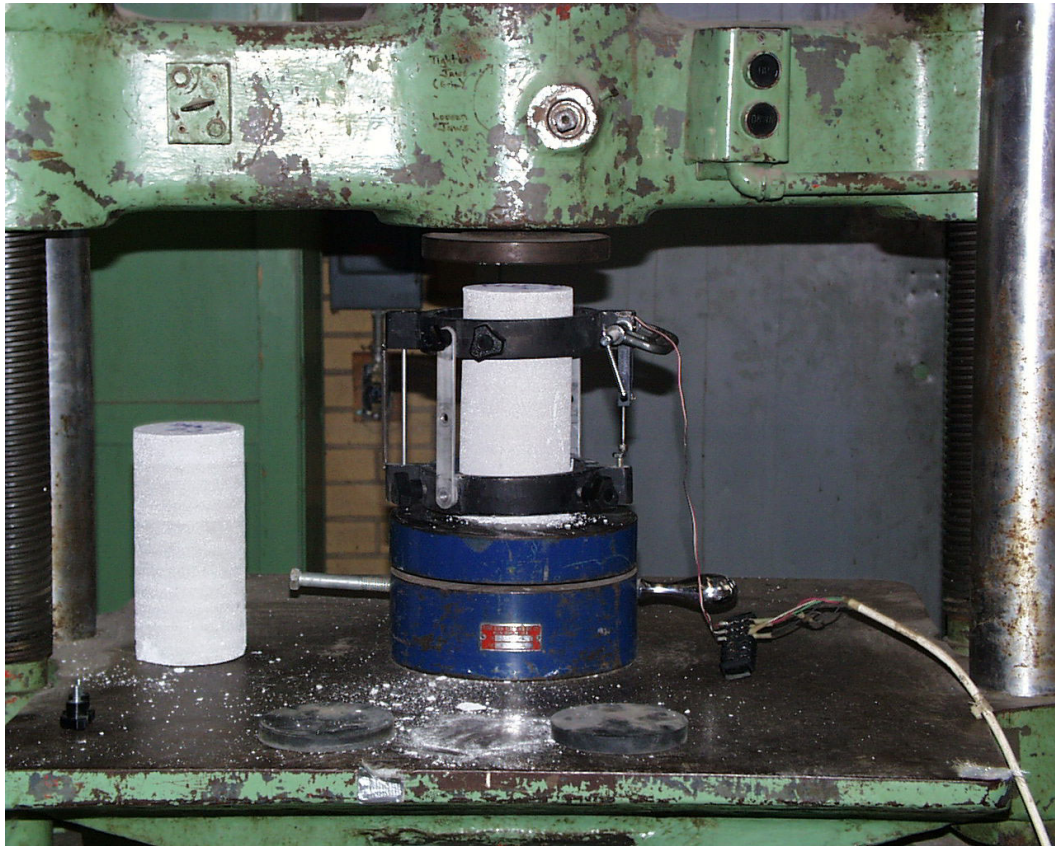
Figure 2.20: Typical view of the test setup to measure compressive strength
