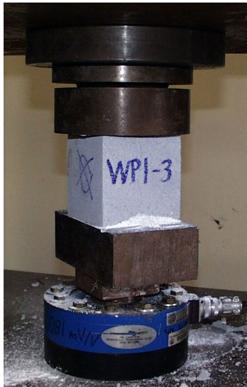
Figure 2.11: Typical view of test setup to measure compressive strength
