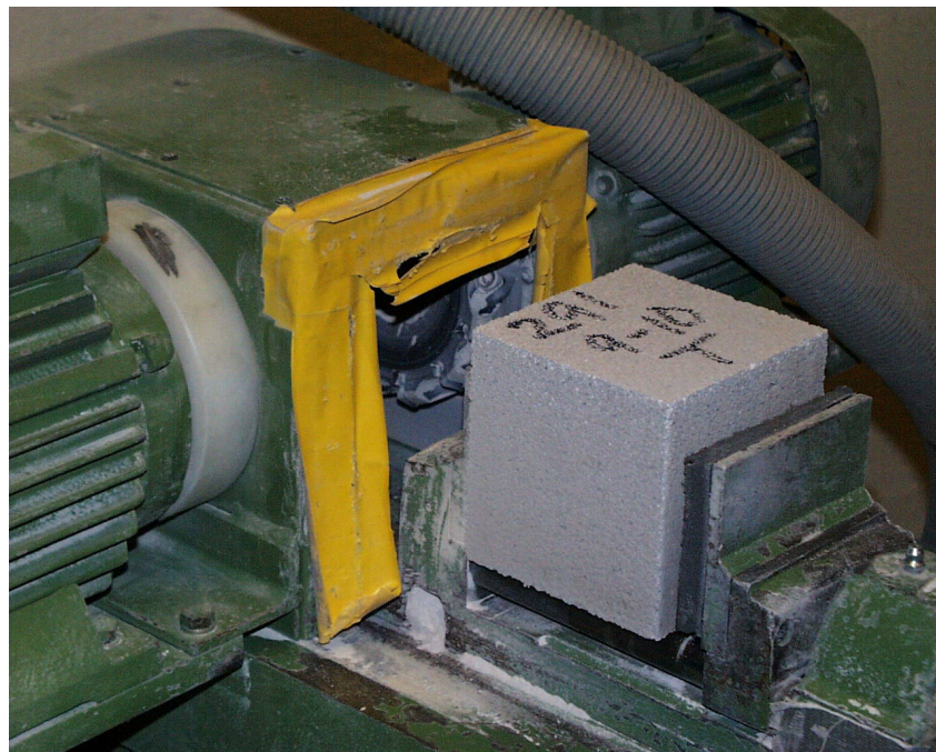
Figure 2.10: Machine used to mill faces of AAC cubes
