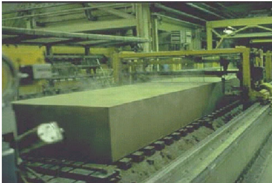
Figure B.4 Fresh AAC after removal of molds
