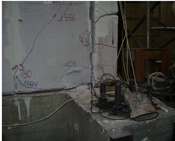
Figure A.35 Loss of end block on compression toe in Shear Wall Specimen 16
